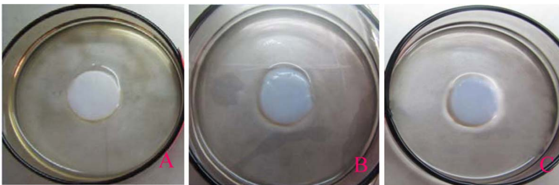
Figure 5. Images of the antibacterial circles of different hydrogels against E. coli : (A) pure PVA, (B) TiO 2 /PVA nanocomposite hydrogel, and (C) TiO 2 /CMCS/PVA nanocomposite hydrogel. [Color figure can be viewed in the online issue, which is available at wileyonlinelibrary.com.]
